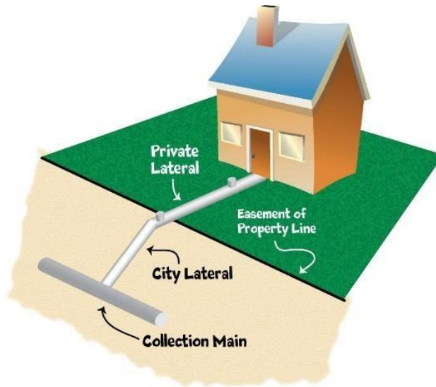
Figure 23 - Private Sewer Lateral Line (COA, n.d., Private Lateral Program)
